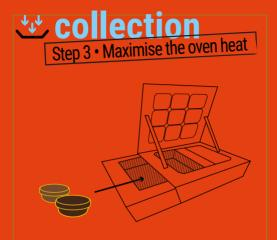
To accumulate a maximum of heat in the oven, the Sunlab is brown. Dark colours have a better absorption capacity of sunrays without send them back, unlike brighter colours.
