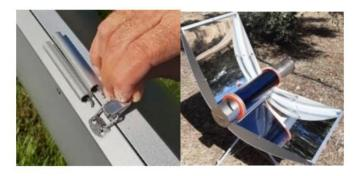
**13.** Tighten the two wing nuts on the right and left to prevent the wing height from to reclose.
