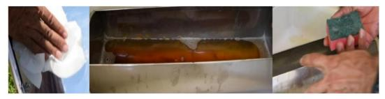
To clean mirrors when they are dusty, always use paper towels dampened with alcohol or window cleaner. Avoid the use of pre-impregnated wipe-type fabrics. Never clean the Pyrex tube when it is hot, only when it is at room temperature.
