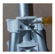
5. Push the tube to align the hole in the tube with the hole in the plastic.
