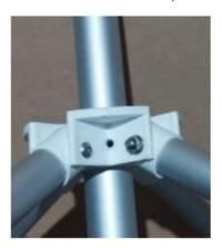
**6.** Replace the nut and screw, and screw them in with the screwdriver. Be careful, if the holes are well aligned you should not have to force to screw.
