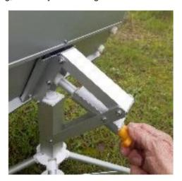
**18.** The SUNCHEF is in the right place horizontally when the shadow cast by the screw at the top of the tube is not visible.
